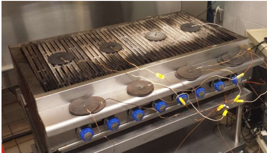
ASTM F1695-03 Section 10.6 Lab Testing Broiler Temperature Measurement
